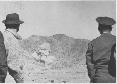
MINIATURE MUSHROOM blossoms as non-nuclear test shot is fired at Coyote Canyon. In preparation for the shot a pit 100 feet long was dug, the rocks removed, and the pit backfilled after pressure gauges were placed in a carefully arranged pattern. Results will show character of shockwave forces moving through the ground.
